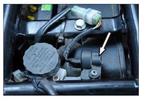
Your motorcycle is fitted with a unique "Roll Over Sensor" under the seat. This is a safety feature.
