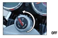
• Turn the ignition key in anticlockwise direction to "OFF". Once you turn off, all the electrical systems goes off. Now the key can be removed.
