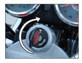
Insert ignition key and turn clockwise direction to "ON". Once you turn on the ignition key all the indicating lights in instrument cluster starts glowing on for few seconds and the engine will get ready to start. The key cannot be removed from "ON" possition.
