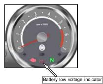
If the battery voltage is less than 12 volts, the low voltage indicator will start glowing continuously.
