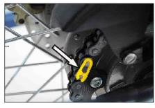
The open end of the chain master link lock should face opposite to normal direction of chain rotation.
