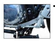
Press the gear pedal upwards with toe to engage 2nd and gear.
