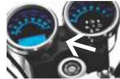
HAZARD SIGNAL BUTTON
